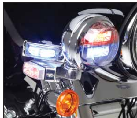
Front passing/fog lamp kit available in 90° or 90° and 45° models. Includes flange.
