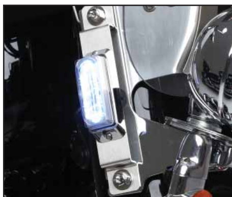
Side Fork Mounting Bracket Kit allows for easy mounting of one lighthouse. Includes flange.
